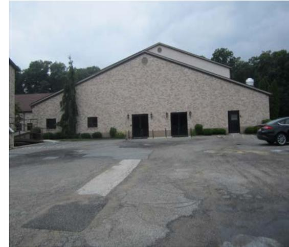
A rain garden can be installed near the shed to the north of the main building and along the western side of the parking lot to capture, treat, and infiltrate stormwater runoff. Porous pavement can be installed in the main parking lot in the southernmost parking spaces to capture and infiltrate runoff from the parking lot. A preliminary soil assessment suggests that the soils have suitable drainage characteristics for green infrastructure.
