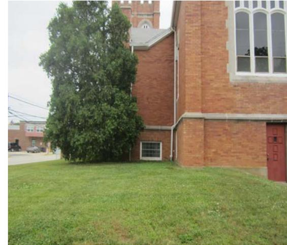
Two twin rain gardens can be installed in the two turfgrass areas in front of the southeast entrance of the church building to capture and infiltrate stormwater runoff from the church roof. A preliminary soil assessment suggests that the soils have suitable drainage characteristics for green infrastructure.
